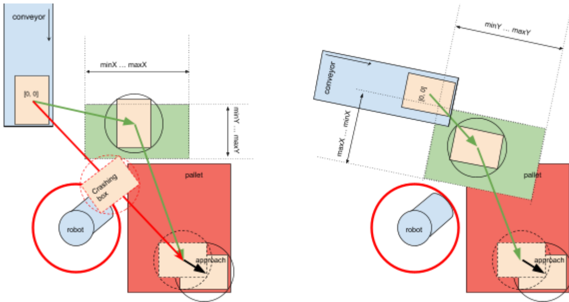
Figure 9: Illustration of the smart exit search area.
